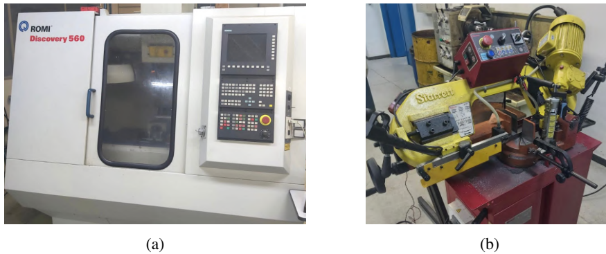
Figure 2: Equipments employed at the MC production: (a) machining center; (b) band saw
